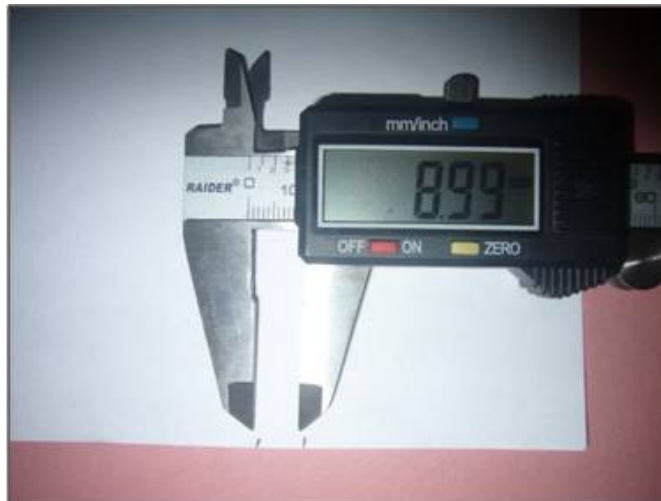
Figure 2: A photograph of an A4 paper, a digital caliper showing how the landmarks were marked (from the radiograph) and measured with the caliper
