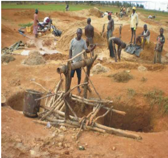
Fig.2: Rudimentary Haulage and tin Processing Technique
