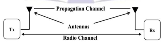
Figure 3: Radio and Propagation Channels (Jinan, 2010).
