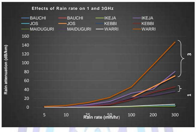
Figure 13: Effects of Rain rate on 1 and 3GHz
