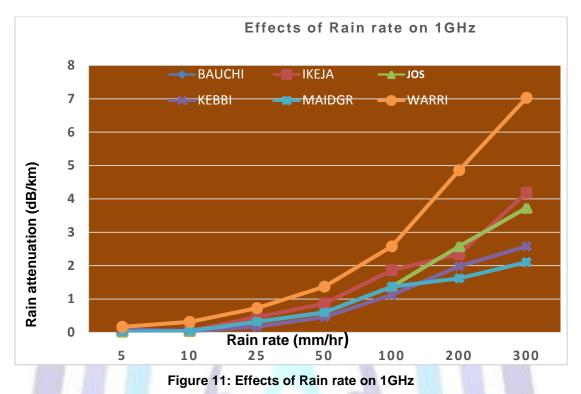
Figure 11 shows that attenuation has less impact on lower frequencies but increase with higher frequencies.
