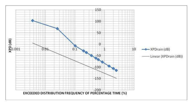
**Figure 3.** Cross Polarization Discrimination (XPD) variation with exceeded distribution frequency of percentage time
