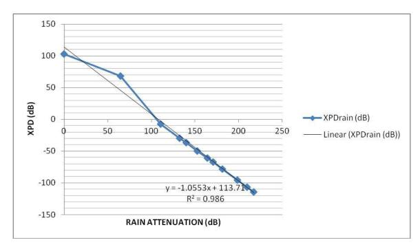
Figure 5: Show Cross Polarization Discrimination (XPD) with Rain Attenuation (C<sub>A</sub>)Relation in Jos.
