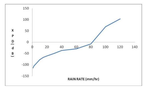
Figure 4. Cross polarization discrimination (XPD) variation against Rain rate.
