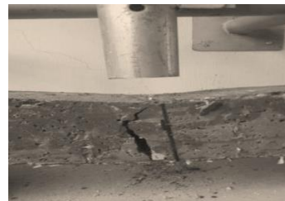
(f) Failure mode of sample with 0.5% fibre and 15% RHA
