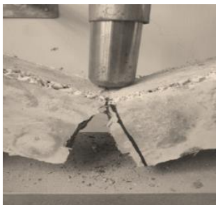
(d) Failure mode of sample with 0% fibre concrete without RHA
