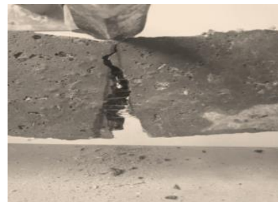
(e) Failure mode of sample with 0.5% fibre and 5% RHA
