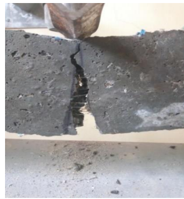
(b) Failure after Impact
