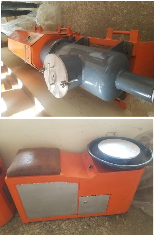
Plate 9: Industrial Throwing Wheel and a Pugmil for Ceramics Constructed by: Staff and Students of Visual Arts Source: Babson Ajibade, 2023
