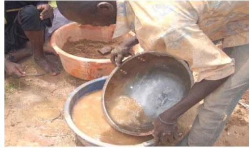
Fig. 9 A process of separating fine gold particles from the gangue minerals after mercury amalgamation.
