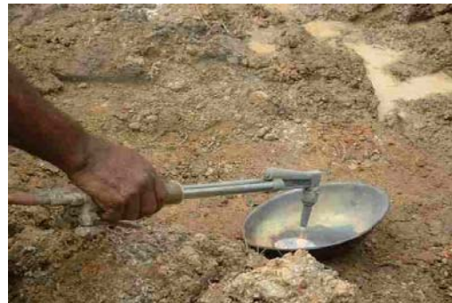
Fig. 10 Burning of mercury amalgam using blow torch to evaporate mercury, leaving gold nuggets.
