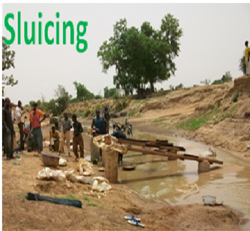
Fig. 7 Washing of ground gold ore material in a sluice box to concentrate gold.
