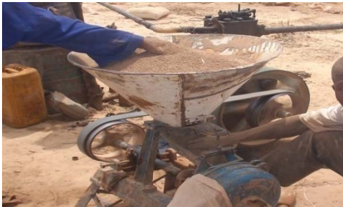
Fig. 6 Local miners using bare hands in grinding of broken gold material into powder (pulverization) using a locally fabricated grinding mill.
